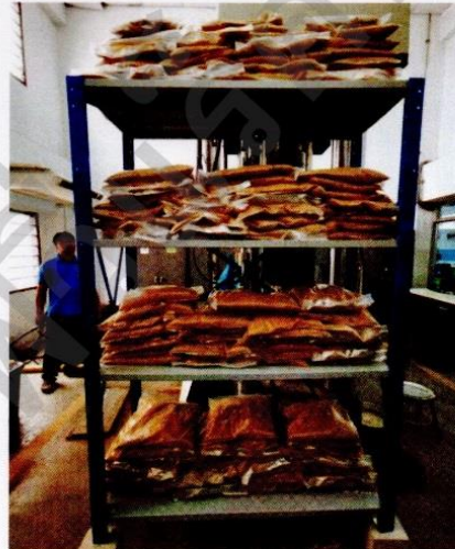
Figure 4 : Testing Configuration (load = 150 kg./layer) on 20 November 2019
