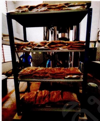
Figure 3 : Testing Configuration (load = 75 kg./layer) on 19 November 2019
