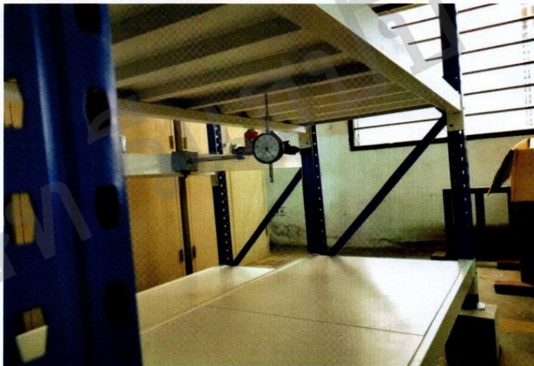
Figure 2 : Measurement of Deflection using Dial Gauge
