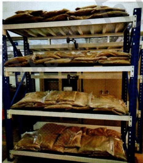
Figure 4 : Testing Configuration (load = 350 kg./layer) on 20 September 2019
