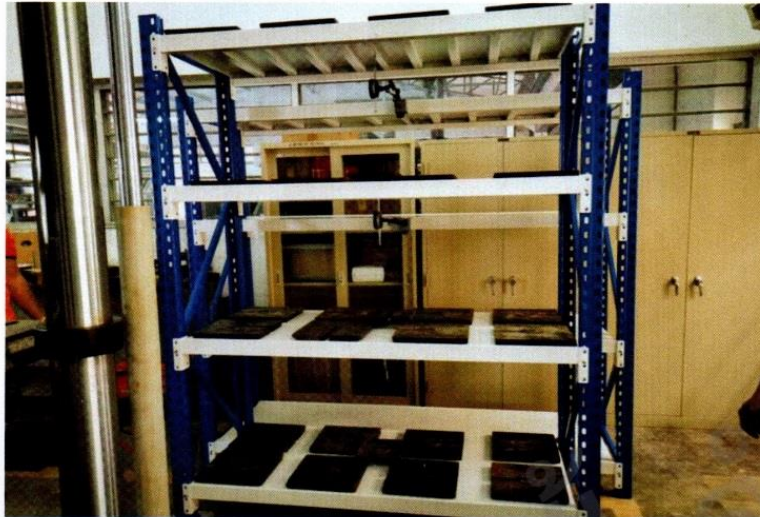
Figure 3 : Testing Configuration (load = 87.5 kg./layer) on 19 September 2019
