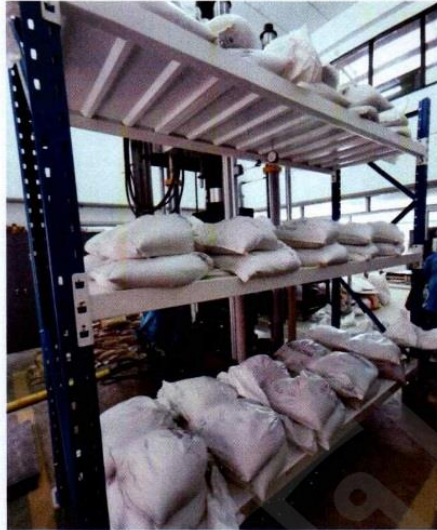
Figure 2 : Testing Configuration (load = 400 kg./layer) on 27 May 2020
