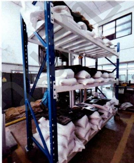
Figure 3 : Testing Configuration (load = 800 kg./layer) on 28 May 2020
