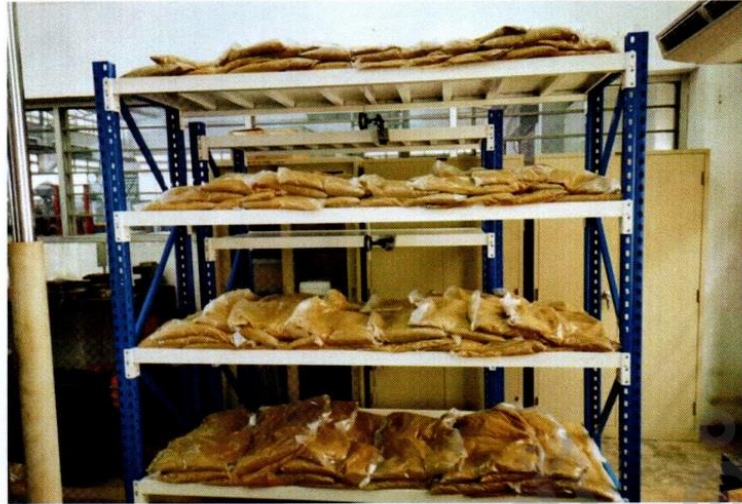
Figure 3 : Testing Configuration (load = 150 kg./layer) on 20 September 2019
