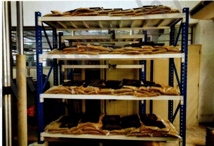
Figure 4 : Testing Configuration (load = 300 kg./layer) on 21 September 2019
